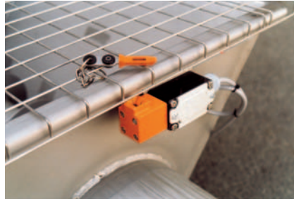
Safety devices fitted with a key system.
