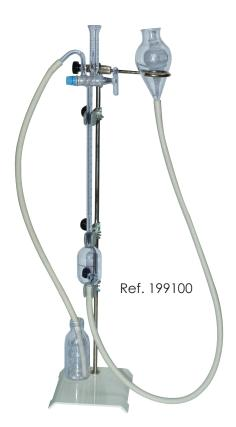
In laboratories, the Van Slyke equipment is used to simply measure the volume in CO2, even lower than 200mg/l, by mercury suction.
